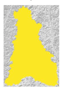
21. To obtain the polygon of the basin, it is only necessary to convert the raster to a polygon type vector (shapefile), this can be done with the **r.to.vect** tool.
